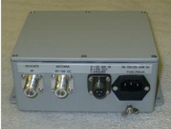
MISC-A0022 wideband 15 V power supply and DC injector suitable for use in conjunction with the OMNI- A0268.
