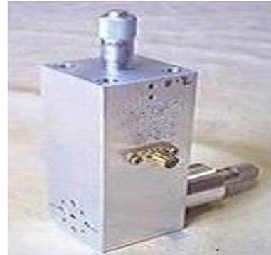
Figure 1. Dual Tuner Gunn Oscillator Module
